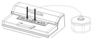
Press the "Vakuumbehälter" (Canister) button to start vacuuming. To ensure there is no air leaking between the cover and the canister, use
