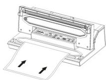
Clean and straighten the open end of the bag--ensure there are no wrinkles or ripples.
