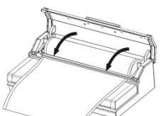
Put down the cutter rack and make sure it is on the right place of the bags, then slide the cutter from one end to the other end to cut the bag.
