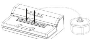
Press the “Vakuumbehälter” (Canister) button to start vacuuming. To ensure there is no air leaking between the cover and the canister, use your hand to push down the cover at the beginning of the vacuuming work. The status Indicator F light. Once it is finished, light will turn off.
