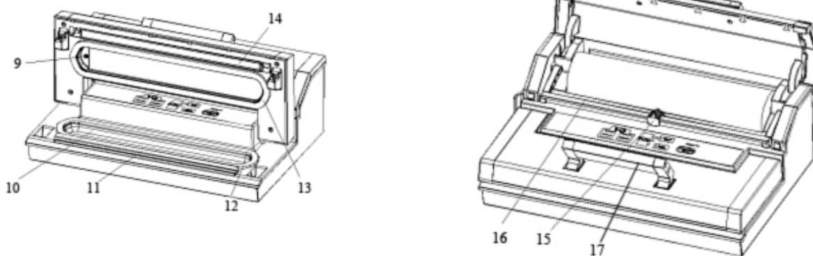
**9. Air intake:** Air intake connects with vacuum chamber and pump. Do not cover this air intake when placing bag for Vacuum&Seal operations.
