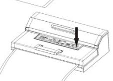
Press "Manuelles Schweißen" (manual seal) button to start sealing the bags. The status Indicator D light. Once it is finished, light will turn off.
