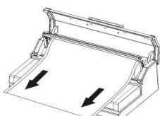
Make sure the bag cutter is on one end of the cutter rack, then put the cutter rack to the back.
