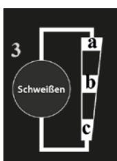
Check the LED status of “sealing time” (a, b, c) to confirm sealing time depending on the moisture status of packed items according to the type of food;
