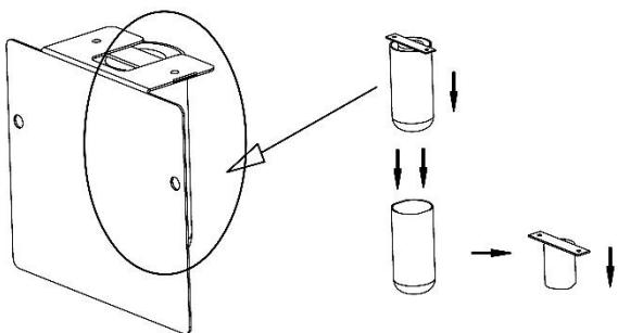
Pull the cover of the UV lamp downwards and replace the lamp.
