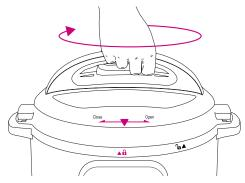
The pressure cooking lid **automatically seals** for easy pressure cooking, but **does not lock into place when closed**. The lid can be removed during Pre-heating but **locks into place once the cooker has pressurised**.
